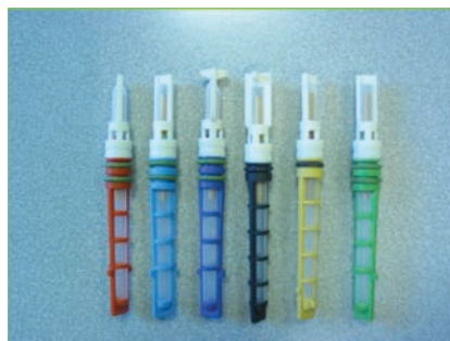
Orifices tubes are colour coded
